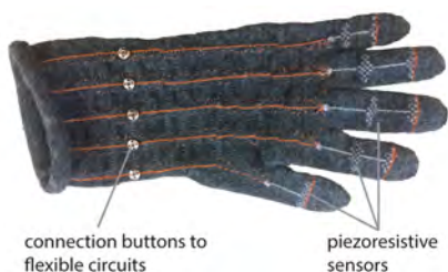
Figure 1. The e-textile glove used in our work. The light grey fibres are piezoresistive fibres. The buttons are sewn on the textiles to connect to the flexible circuit board.
