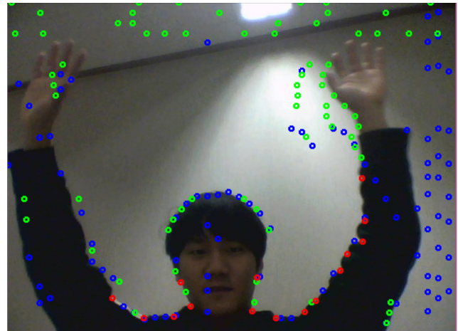
Figure 2. Harris corner detection on a frame in three orthogonal planes, (x,y) , (x,t) , and (y,t) [red = (x,y) , green = (x,t) , blue = (y,t) ].
