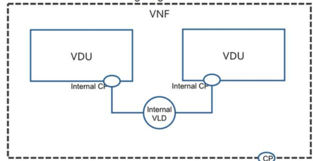
Figure 1 Virtual Network Function Descriptor [7]
