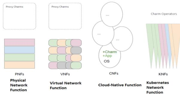
Figure 3. Generation of Network Function with OSM [7]
