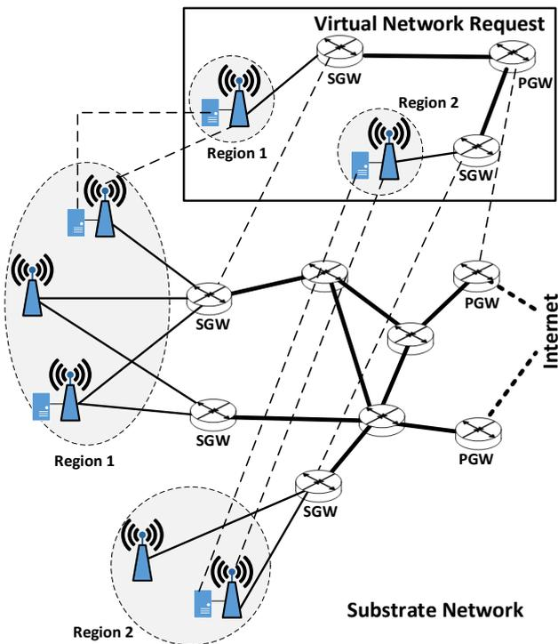
Fig. 3: Embedding of Mobile Edge Computing Networks
