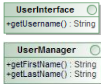
Figure 4. Example of two interface requiring Different Control Structures.
