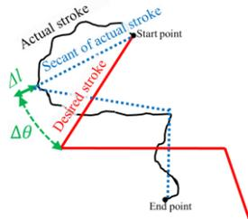
Figure 7. Evaluation values: the differences of lengths and angles between the secants of actual trajectory and the desired trajectory
