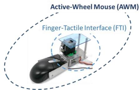
Figure 1. Active wheel mouse (AWM): the finger-tactile interface (FTI) is attached at the front
