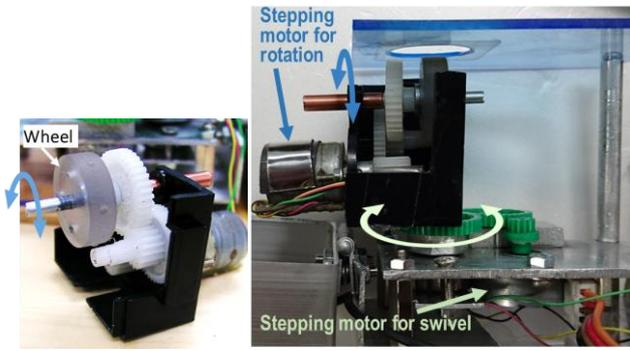
(a) Rotation mechanism (b) Finger-tactile interface in total
